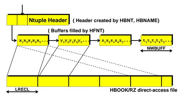
Figure 3.2: Schematic structure of a CWN Ntuple
