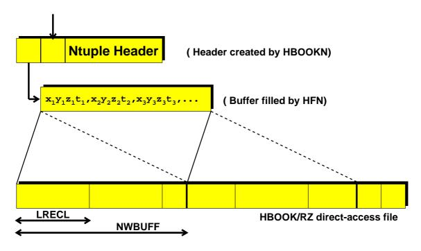
Figure 3.1: Schematic structure of a RWN Ntuple
